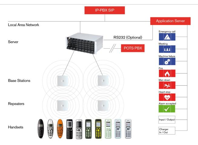
up to 8 base stations, and each KIRK Base Station is able to connect with up to 3 KIRK Repeaters. The KIRK Wireless Server 8000 with analogue interface supports up to 1024 simultaneous calls.
