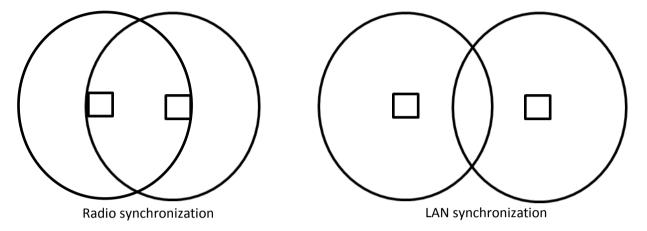
It should be noted that depending on the deployment - synchronization via LAN and radio can be combined in the same DECT installation. Even when a base station is configured to synchronize via LAN, it transmits the signal required for synchronization via radio. Therefore, base stations synchronizing via radio can retrieve their synchronization signal from a base station synchronizing via LAN. The other way around is not possible.
