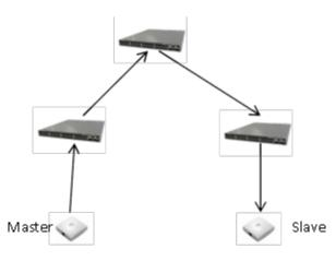
Note: In the lab, the IP-DECT base stations have successfully been synchronized with 5 LAN switches between master and slave.
