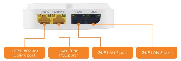
\*PoE PSE port won't supply power (5 W) when the AP is powered by 30 W passive PoE injector.
