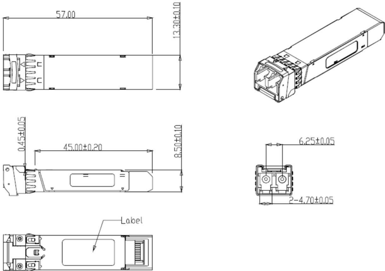
Figure5. Mechanical Specifications
