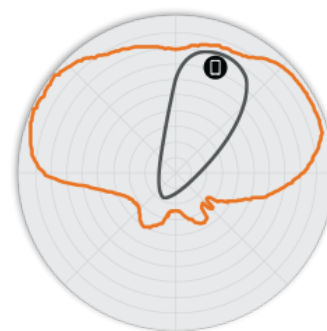
Figure 5. R710 5GHz Elevation Antenna Patterns
