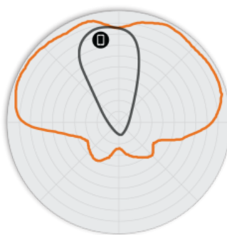
Figure 4. R710 2.4GHz Elevation Antenna Patterns
