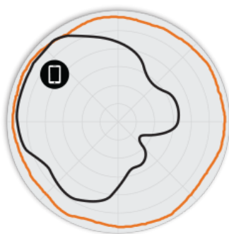
Figure 3. R710 5GHz Azimuth Antenna Patterns
