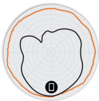
Figure 2. R710 2.4GHz Azimuth Antenna Patterns
