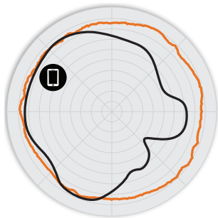
Figure 2. R310 2.4GHz Azimuth Antenna Patterns
